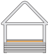
Sub-floor with timber battens
